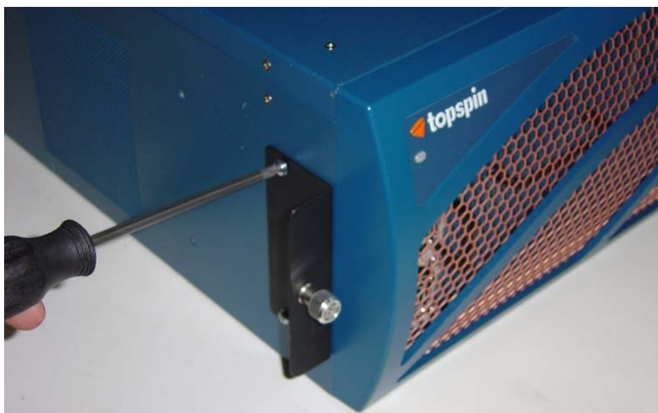
Figure 3-2: Fastening the Side Flanges
